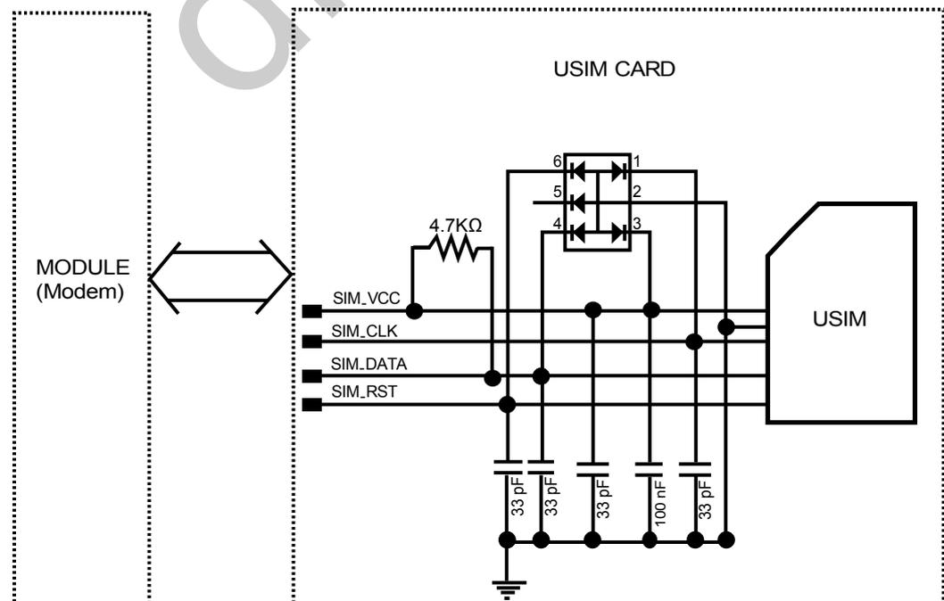
**Figure 3-16** Pin definition of USIM Socket
