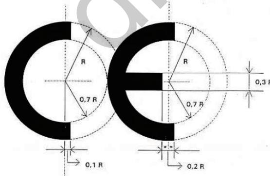
The CE mark of wireless equipment relates to the used frequency bands and the notified body. For this reason, the CE mark on the nameplate consists of letters C and E, the identification number of the notified body, and a ⓘ symbol.
