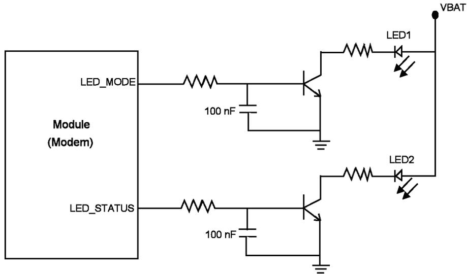
The brightness of the LED depends on the current value, and for most of the indicator lights the current from 2 mA to 5 mA is already enough.
